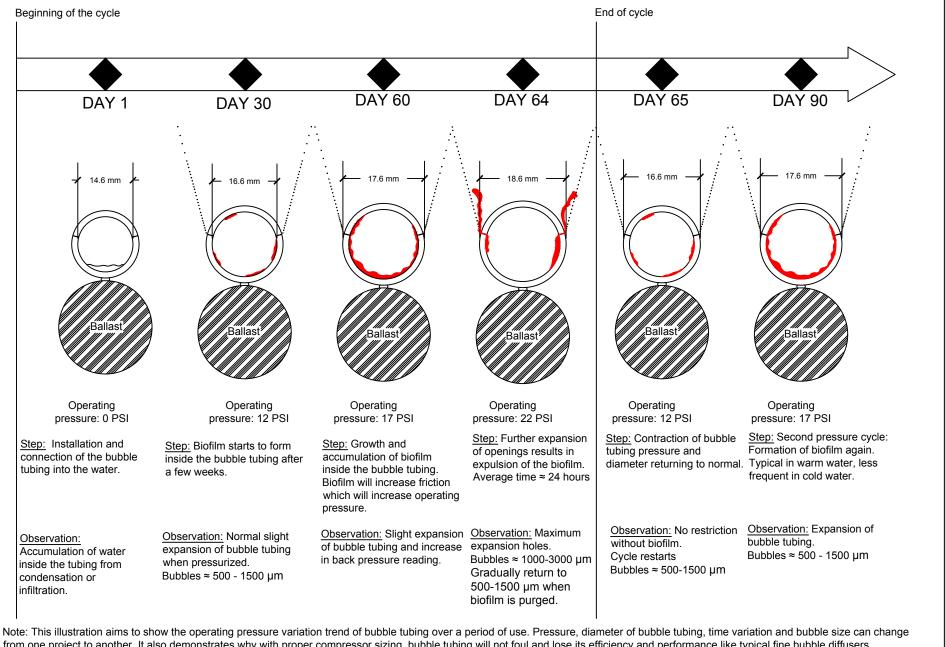
from one project to another. It also demonstrates why with proper compressor sizing, bubble tubing will not foul and lose its efficiency and performance like typical fine bubble diffusers.
